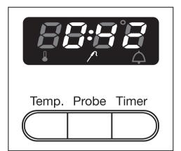
Once the oven has monitored the cooking process, it will only calculate and display the remaining cooking time. From this point on, the core temperature can no longer be displayed.
